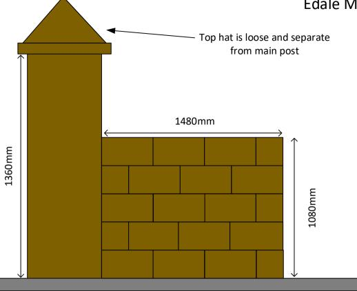
Illustrations are for dimensional purposes only. The dry stone wall will be reconstructed from photographs taken of the post and wall, any major masonry will be put back in its original position
